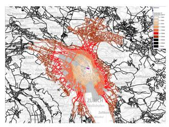
How much potential is there in the vicinity of the railway station? What is the corresponding demand for bicycle parking? This is shown by the isochrone calculation for bicycles at Zurich main sta-tion (Source: developed by EBP using NPVM data).
