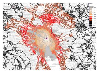
e-bikes extend the catchment area and make the station accessible to more people. This is shown by the isochrone calculation for e-bikes at Zurich Main Station (source: EBP graphic from NPVM ap-plication).
